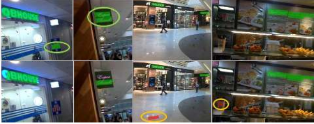
Figure 4: CharNet improves both recall and precision on text detection by jointly learning with character recognition.
