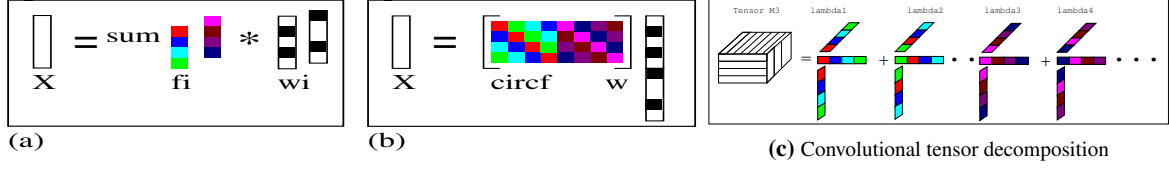
Figure 1: Convolutional tensor decomposition for learning convolutional ICA models. (a) The convolutional generative model with 2 filters. (b) Reformulated model where \mathcal{F}^* is column-stacked circulant matrix. (c) The third order cumulant is decomposed as filters.
