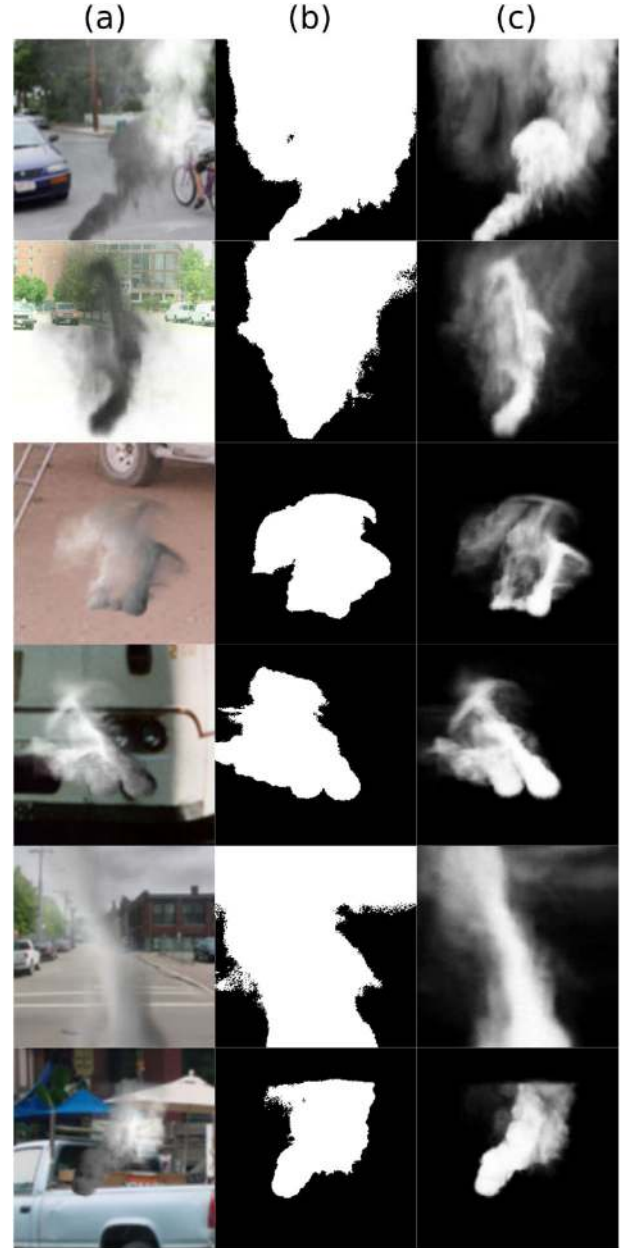
FIGURE 17 (a) Examples of Synthetic RGB images 256 \times 256 pixels of the Yuan test datasets (DS01, DS02 and DS03). (b) Smoke masks generated with threshold 20. (c) Synthetic smoke: Ground truth of alpha channels
