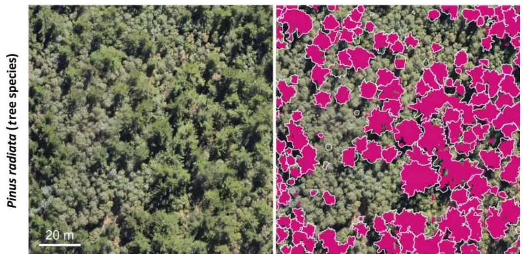
Figure 4. Mapping of the tree species Pinus radiata in central Chile. Left: The input RGB imagery used for the CNN-based segmentation. Right: The reference data (white polygons) and the segmentation results (purple). Centre coordinates: 208876, 6082517, EPSG 32719.
