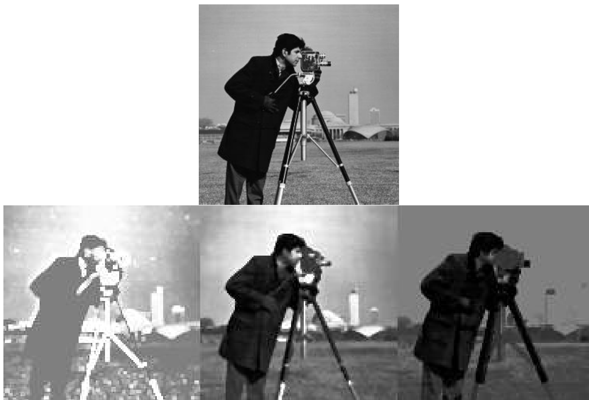
Figure 2.2: At the bottom of the figure are Max, Median and Min (rank) features respectively on the “cameraman”. We see on the bottom left that the max filter dilates high values and contracts low intensity values if they are next to a high one. Median filters acts similarly and dilates median values over others locally but to a lesser degree than the extreme value filters. Note that edges can be found if we use for example a range filter, i.e. Max-Min. Note that we scaled the images below to exaggerate the intensities for display purposes.
