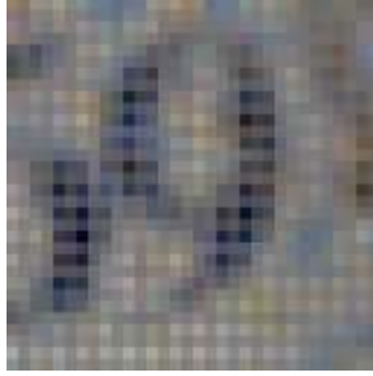
Figure 4.11: Shallow denoising rank transpose autoencoder without overlap scaling. The output had a rank transpose with FoV= 3 \times 3 with a stride \Delta = 2 . Since 3 and 2 are coprime, there is a checkerboard artifact.
