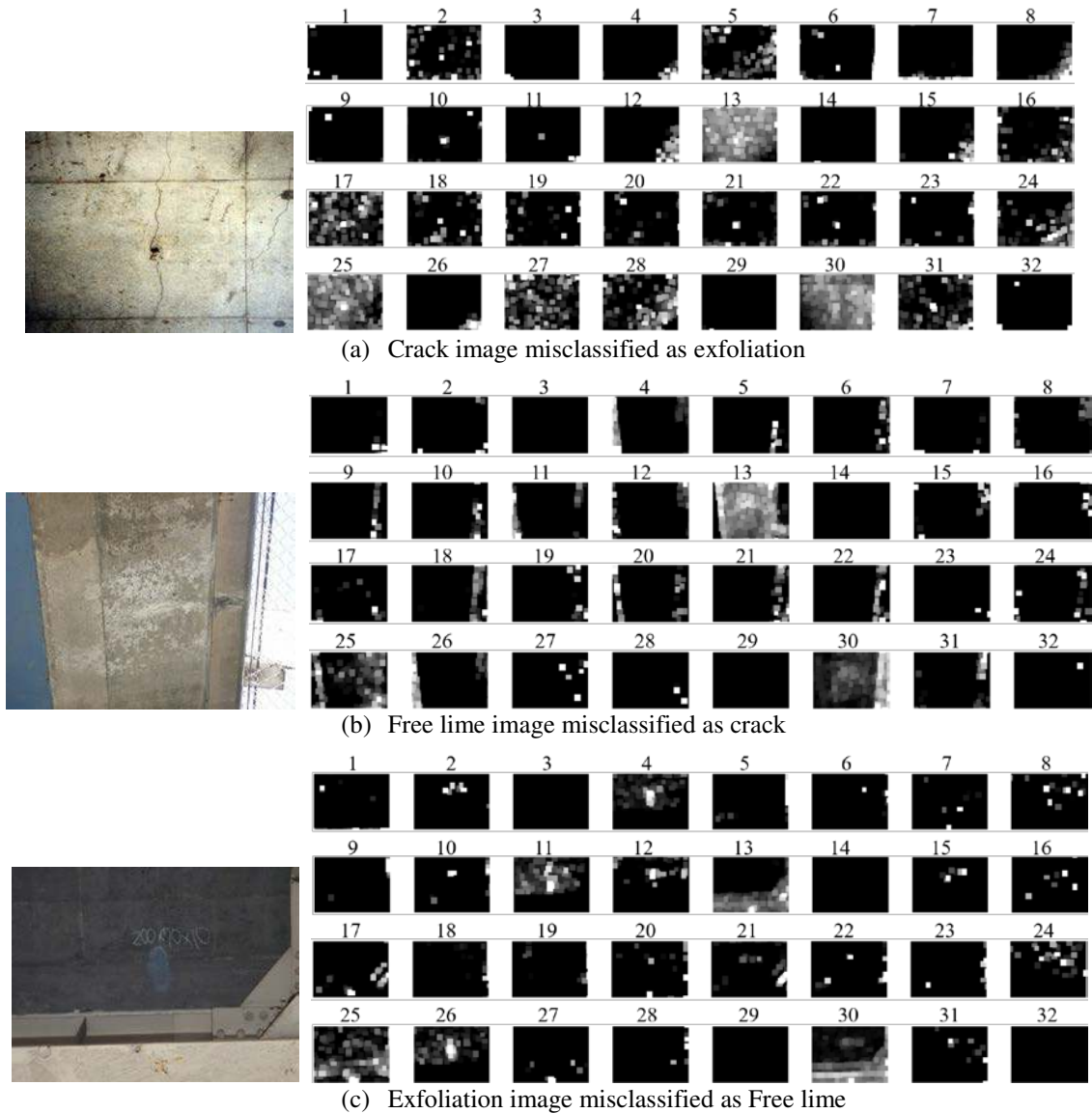
Figure 8 Examples of misclassified test images. Original images (left column) and their corresponding feature maps calculated via the second LRN layer (right column).
