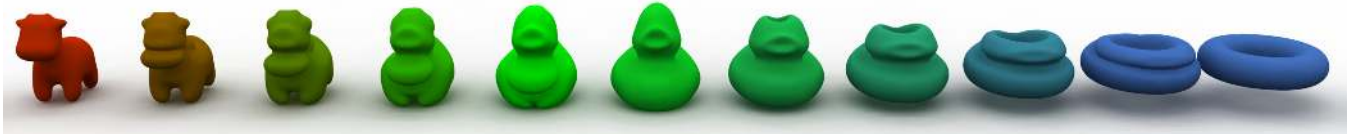
Figure 1: Shape interpolation from a cow to a duck to a torus via convolutional Wasserstein barycenters on a 100 \times 100 \times 100 grid, using the method at the beginning of §7.
