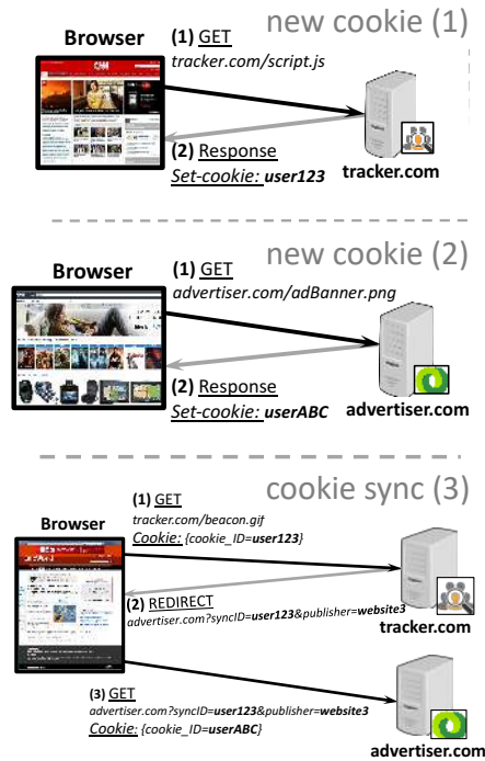
Figure 1: Example of advertiser.com and tracker.com synchronizing their cookieIDs. Interestingly, and without having any code in website3 , advertiser.com learns that: (i) cookieIDs userABC==user123 and (ii) userABC has just visited the given website. Finally, both domains can conduct server-to-server user data merges.
