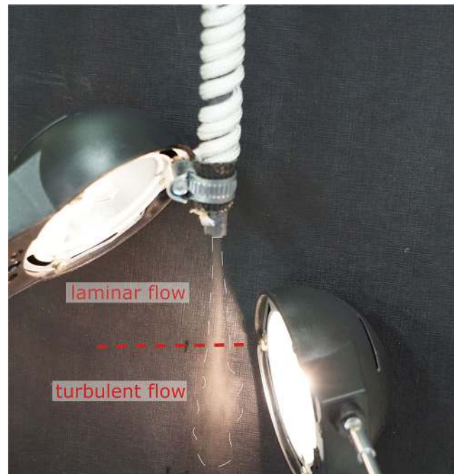
Fig. 10 Photograph of the flow of the nebulized mist from the nozzle, showing a laminar and turbulent flow regime. The flow of nebulized mixture was visualized, as a faint translucent flow, by turning the rope heater off while illuminated the flow from the side, a configuration that enables direct optimization of the specimen-to-nozzle distance in order to position the specimen in the center of the turbulent flow regime
