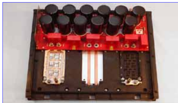
Figure 2: IGBT power semiconductor module (1200V 450A)
