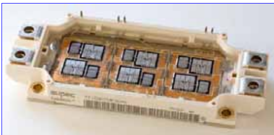
Figure 2: IGBT power semiconductor module (1200V 450A)
