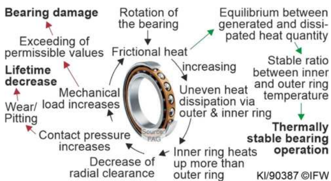
Fig. 11 Tribologically induced reduction of bearing life of rolling bearings according to [82]
