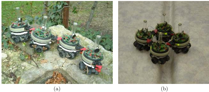
Fig. 1. A group of robots physically connected to each other, that (a) moves on rough terrain. This picture is demonstrative of the capabilities of the self-assembling robots we developed; (b) passes over a gap during an experiment in a close arena with a flat terrain.
