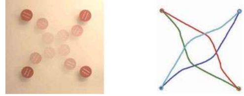
Fig. 11. Experiment with four e-puck robots exchanging antipodal positions. Time-lapse and trajectories. Trajectories are smooth and collision-free.
