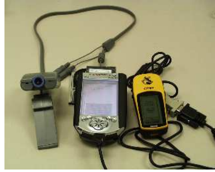
Figure 9: Prototype Node with Video Camera and GPS Receiver Attached
