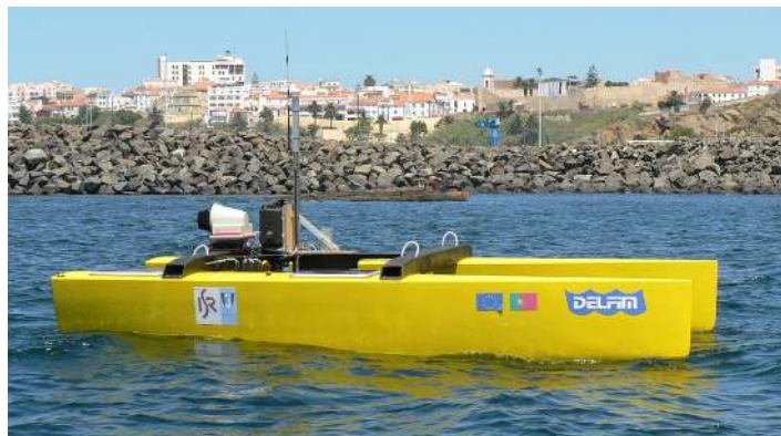
Figure 1. The DELFIMx autonomous catamaran.
