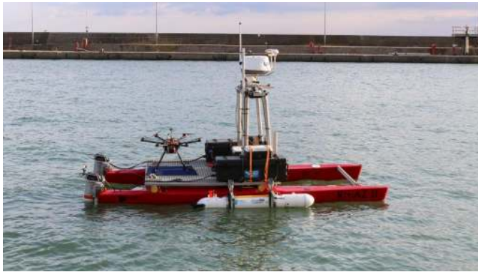
Fig. 2. Roaz carrying the MARES AUV during "euRathlon 2015", in Italy.
