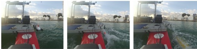
Fig. 3. Sequence of pictures during the deployment of the MARES AUV from Roaz ASV.
