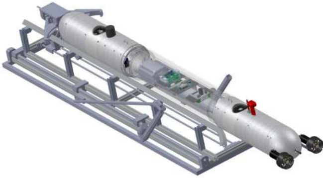
Fig. 6. Schematic overview of the LARS for the DART AUV, in a retracted position. The LARS is actuated to extend and rotate the cradle so that the AUV slides into the water tail-first.
