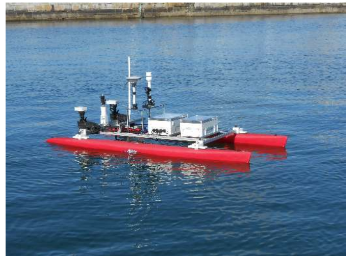
Fig. 5. Zarco ASV with 2.7m long pontoons.
