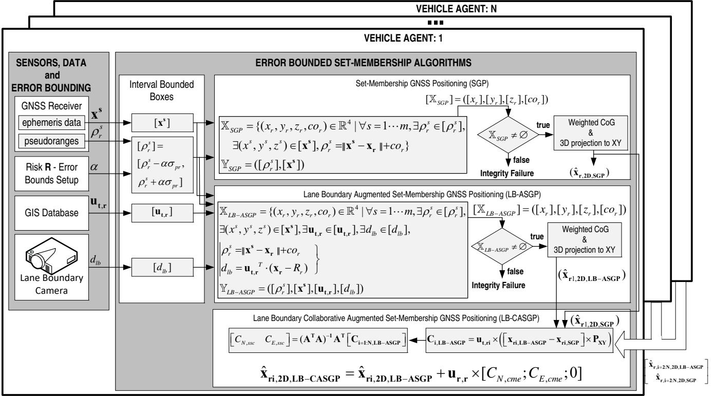
Figure 3: Dataflow and LB-CASGP algorithm architecture.
