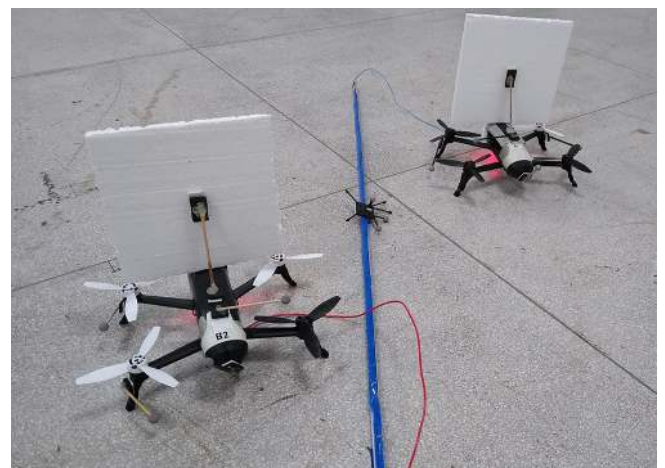
FIGURE 8. Experimental setup containing the used quadrotors, bar-shaped payload, and drag foam plates.
