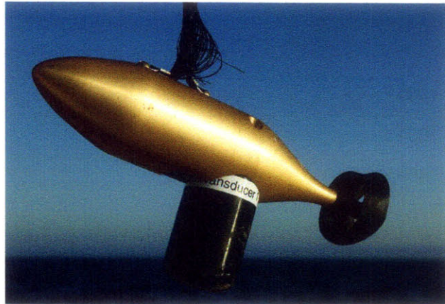
(b) Towfish with modem transducer
