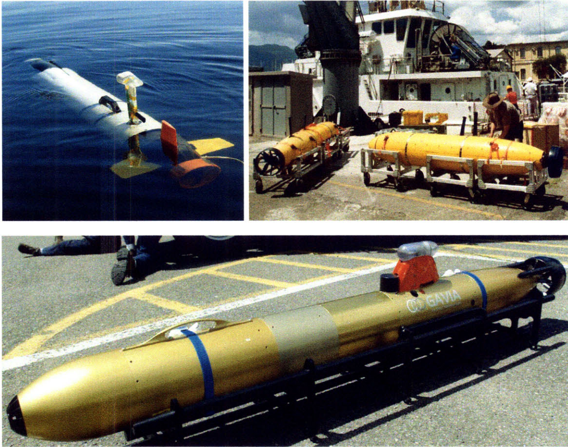
Figure 1-2: Various torpedo-shaped AUVs. Top left: the low-cost, “human-portable” IVER from Ocean Server. Top right: two Bluefin21 prior to being loaded onto the Leonardo during the GOATS04 experiment. Bottom row: the Gavia AUV made by Hafmynd.
