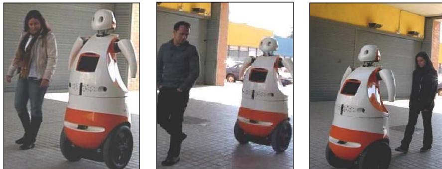
Figure 8: Three different people walking with Tibi Robot. Left: Tibi walks side by side with the volunteer. Center: Robot walks behind the person pushing him/her (the Helbings' pushing force is applied). Right: Tibi walks in front of the person and, here, the dragging force is applied.
