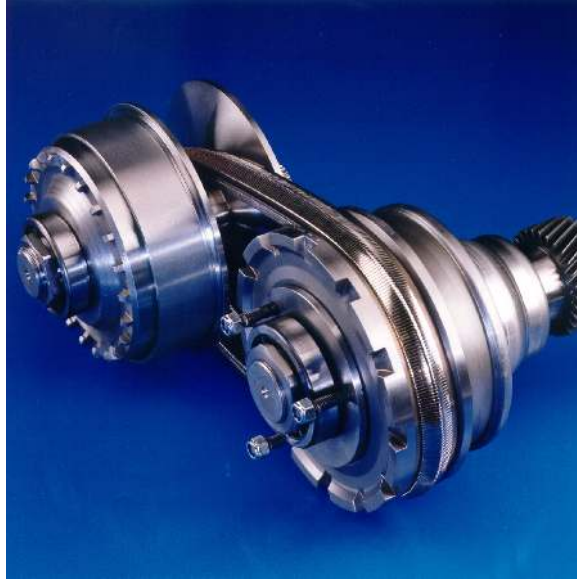
Figure 6.4: Picture of a variator by Van Doorne's Transmissie
