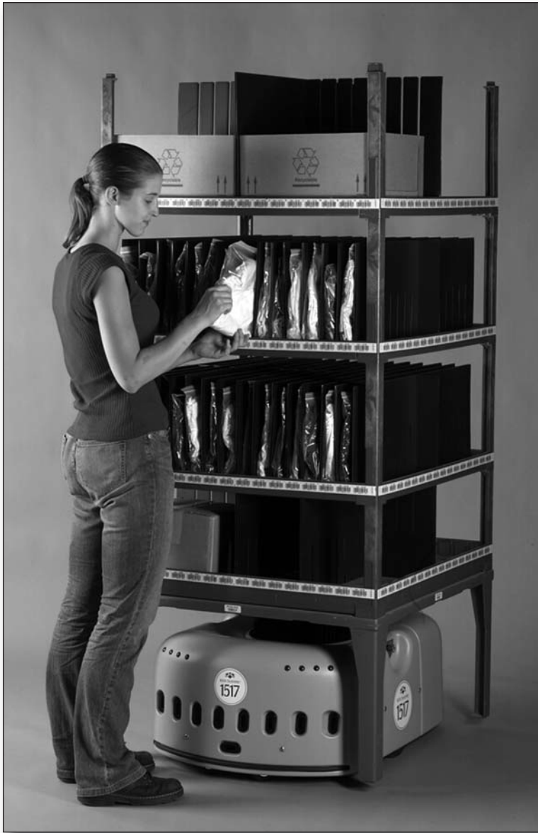
Figure 2. A Kiva Drive Unit and Storage Pod.
