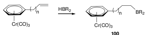
Scheme 19. Formation of 100 by hydroboration, where n = 1 or 2 and \text{HBR}_2 = \text{HB}(1,2\text{-O}_2\text{C}_6\text{H}_4) (catecholborane), \text{HBC}_8\text{H}_{14} (BBN), and \text{HBR}_2\cdot\text{SMe}_2 .
