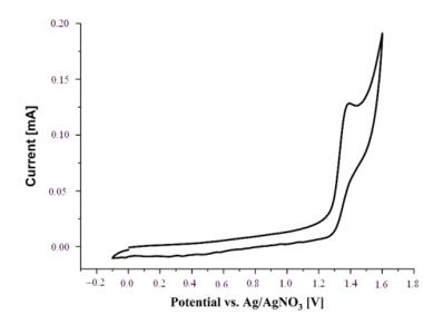
**Figure 1.** CV curve of crystalline **6** (0.1 mM) in MeCN at 25 °C (0.1M [NBu<sub>4</sub>][PF<sub>6</sub>] supporting electrolyte; scan rate 100 mV s<sup>-1</sup>; Pt-wire as working electrode, Ag/AgNO<sub>3</sub> as reference electrode.
