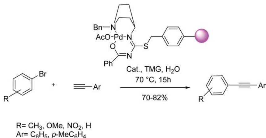
Scheme 30 Copper-free Sonogashira coupling reactions in the presence of the 3-benzoyl-1-(1-benzylpiperidin-4-yl)-2-thiopseudourea-Pd(II).
