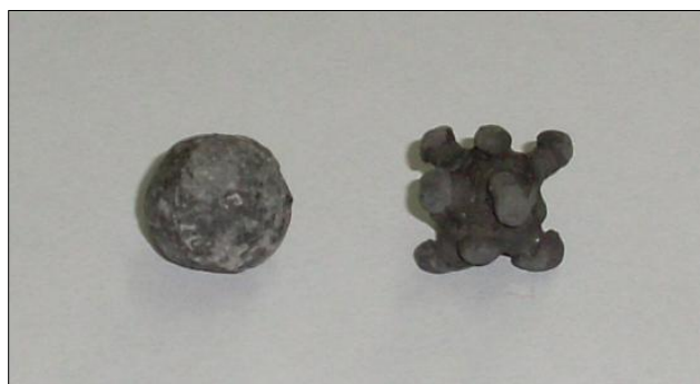
FIGURE 3. Triazole Products Covered with CuNPs/C [ ca. 8 mm (left) and 10 mm (right)] (Reproduced from Ref. 27b with Permission from The Royal Society of Chemistry).
