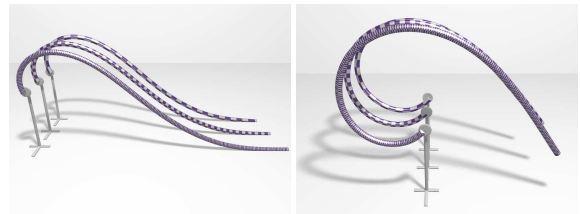
Figure 5: Coiling up three clamped rods. The rods are discretized into 1000, 100 and 50 elements, illustrating that the global deformation is independent of the discretization.
