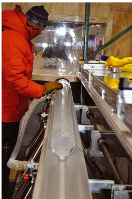
Fig. 5. A run of ice core is coming out of the FED and into the 4 m push-out tray at the 'Receiving and logging' station. On the other side of the wooden wall is the drilling arch.
