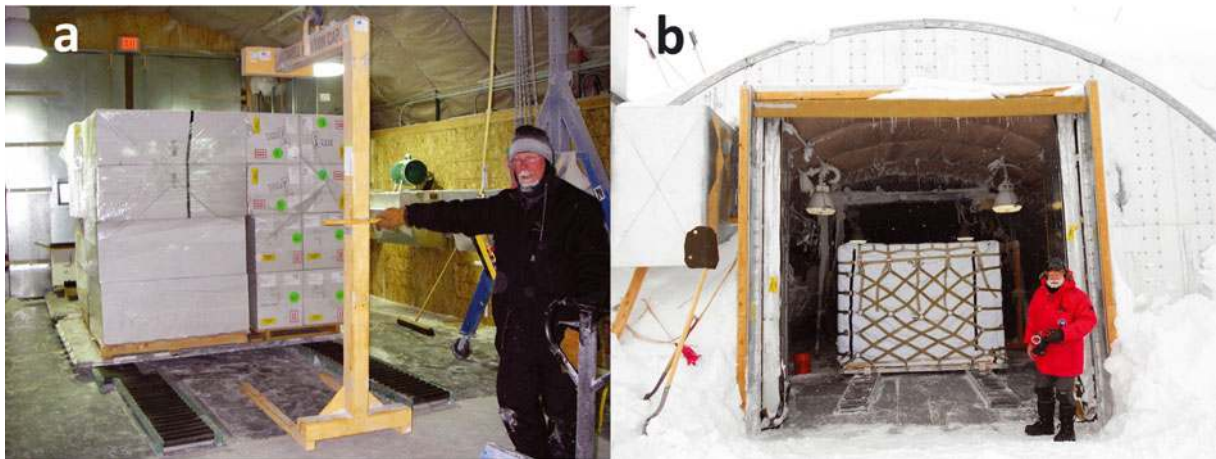
Fig. 7. (a) View of the inside of the core-handling arch showing an AFP with four wood skids (32 ISC boxes) of ice core. Also shown is the roller track system on the floor to facilitate the movement of the AFPs. (b) A finished AFP of ice cores sits inside the core-handling arch as it waits for its cold-deck LC-130 flight to McMurdo Station.
