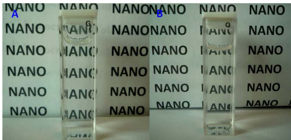
Figure 5. Photographic images of (A) oleate-capped (NaGdF 4 :3% Nd 3+ )/NaGdF 4 nanocrystals dispersed in hexane and (B) ligand-free (NaGdF 4 :3% Nd 3+ )/NaGdF 4 nanocrystals dispersed in water.
