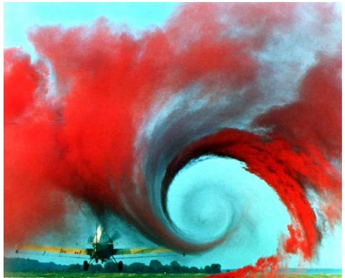
Fig. 1. Wake vortex study from NASA Langley Research Center [9]. The flow around a starting agricultural plane is made visible using smoke injection. A huge pattern of swirling particle motion is created by the aircraft's wake vortex. This paper aims at extracting the cores of such areas.
