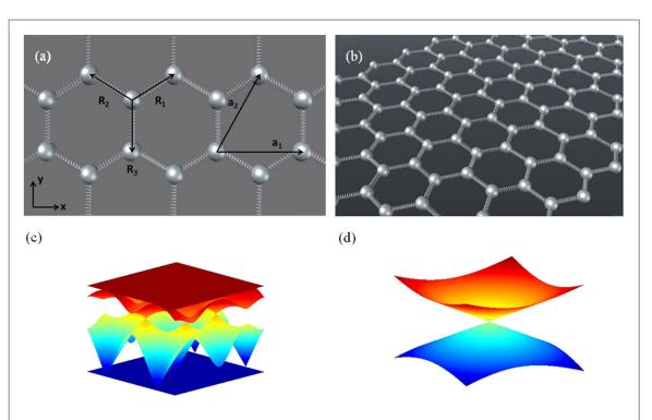
**Figure 1.** (a) Top view of our model made by soft springs and rigid particles. (b) A three-dimensional plot of the semi-infinite mass-spring ribbon ending with zigzag edges. (c) The band structure of two-dimensional mass-spring model with honeycomb lattice and (d) a zoomed-in figure of Dirac cone in the vicinity of a certain K point with mass and elastic constant equals to ten grams and  $4 \text{ N m}^{-1}$ , respectively.
