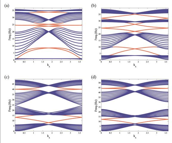
**Figure 4.** Frequency diagram in one dimension for a mass-spring ribbon end with bearded boundary applied constantly angular velocity at (a)  $\Omega = 1$ , (b)  $\Omega = 4$ , (c)  $\Omega = \Omega_c$ , and (d)  $\Omega = 15$  Hertz.
