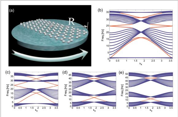
**Figure 3.** (a) A schematic diagram of the non-inertial system. One-dimensional band structure for a mass-spring ribbon end with zigzag boundary applied constantly angular velocity (b)  $\Omega = 1$ , (c)  $\Omega = 4$ , (d)  $\Omega = \Omega_c$ , and (e)  $\Omega = 15$  Hertz.
