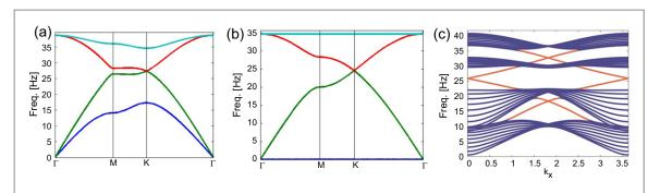
**Figure A1.** The band structure with different transverse constant (a) 1 (b) 0. Red and green line denote optical and acoustic longitudinal modes, respectively; light blue and blue represent transverse modes. (c) The effect of considering transverse elastic constant  $C_T = 0.5$  [N m<sup>-1</sup>]. The first band gap is closed and the others decrease as  $\Omega = 4$  [Hz].
