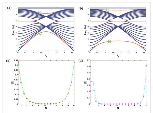
**Figure 2.** (a) The one-dimensional band diagram calculated from zigzag spring-mass ribbon. (b) One-dimensional band diagram for bearded edges. (c) Absolute value of amplitudes for zigzag edge modes, the green dashed line corresponds to the top edge state and the red circles are to the opposite one. (d) Its absolute value of amplitudes of figure 2(b) for both edge states.
