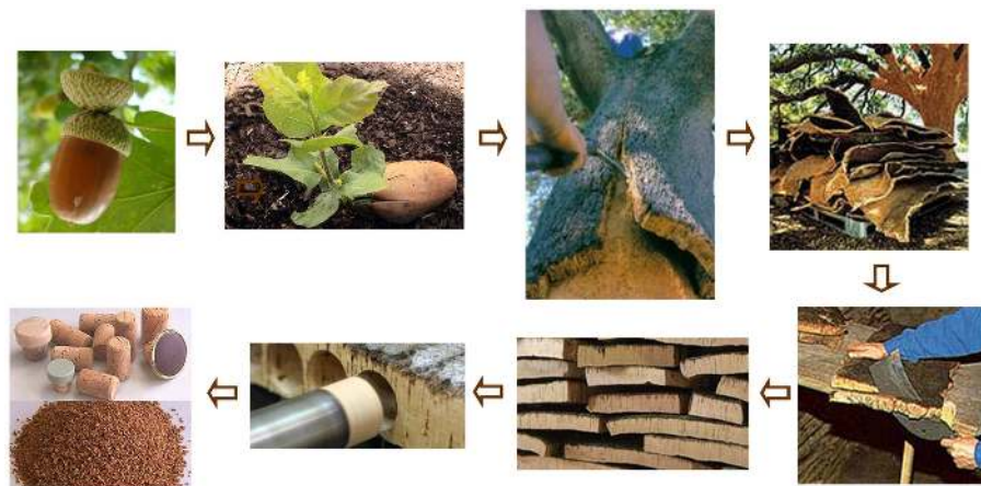
FIGURE 4 | From the cork oak ( Quercus suber L. ) to natural cork stoppers and cork granulates.
