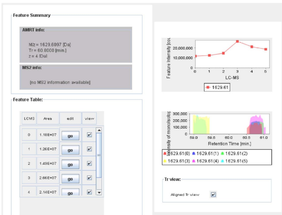
Figure 4 APML viewer. Corra also provides a 2D graphical APML viewer, for user-friendly visualization of peak list or aligned APML files. A) It allows for color-coding of displayed features according to observed charge state, or the number of LC-MS runs the feature was successfully aligned for. Feature coordinates can be zoomed in and out to allow viewing of entire APML files, or just regions of particular interest. B) When a given aligned feature is selected, a pop-up window will be displayed for that feature across all LC-MS runs in the dataset.
