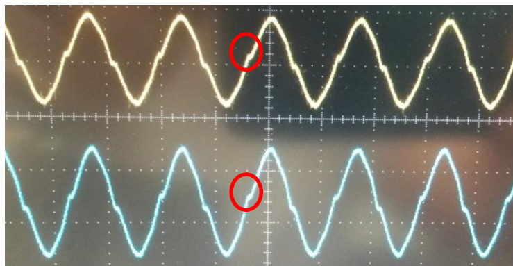
Figure 6-11. Unipolar inverter output distortion due to dead time
