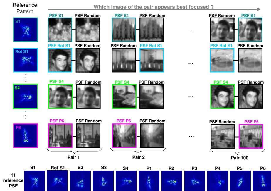
Figure 8.5: Sequence of images in the 2AFC procedure of Experiment 2 (in which images were blurred by different HOA but with the same SR as the subject's natural PSF, shown here for subject S1). In each pair, one of the images was always blurred with a constant reference PSF, while the other was blurred with a randomly selected PSF. The 11 reference PSFs corresponded to the PSF of the subject, a rotated version of their PSF, the PSFs for the three remaining subjects, and six other PSFs from the database. One-hundred image pairs were shown for each reference (corresponding to the 10 images in Figure 8.1, each shown 10 times in random order).
