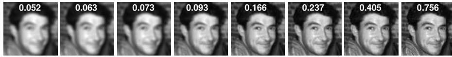
Figure 8.2: Subset of images used in the first experiment (from a total of 128 images). Images are blurred by defocus (the corresponding Strehl Ratios are marked in white).
