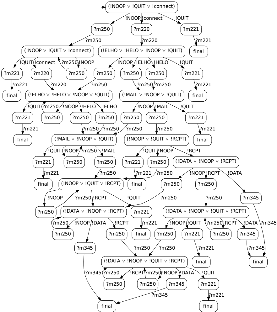
Figure 2.5: Operating guideline for the SMTP protocol (reduced version) as calculated by the tool Wendy.
