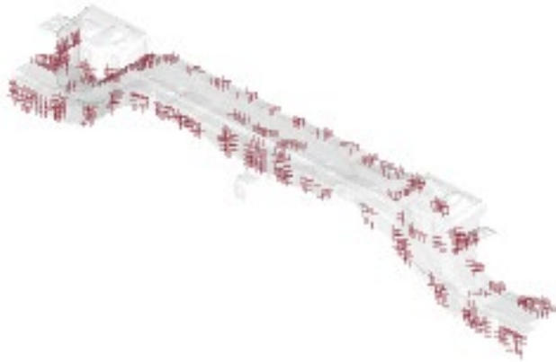
Figure 9. Contact Interfaces of car front-end module
