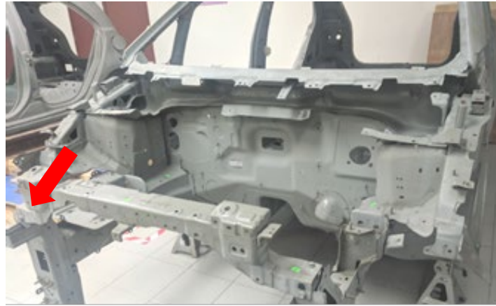
Figure 1. The front-end module of a car body in white.
