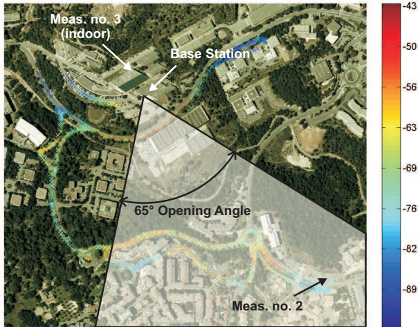
Fig. 3. Map of the measurement scenario. The position and the opening angle of the BS antenna are also indicated. In the first measurement the users were driving in cars along the indicated routes (the colors show the received signal strength in dBm along the routes). In the second and third measurement the users were close together at the indicated positions.
