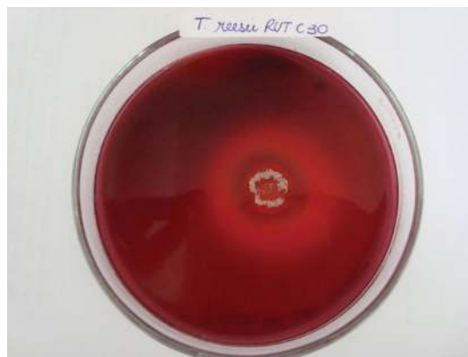
FIGURE 1: Observation of the clear zone around a colony of T. reesei Rut C30 using Congo red dye.
