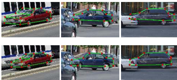
Figure 1. A comparison between two different appearance models used with the same shape model for the task of car alignment. Top Row: car alignment with a random forest based landmark appearance model. Bottom Row: car alignment with the proposed landmark detector.
