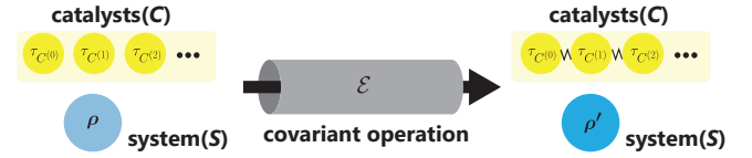
FIG. 1. Schematic of marginal-catalytic covariant transformations. Each catalyst should get back to the original state, while it can correlate with the system and other catalysts.
