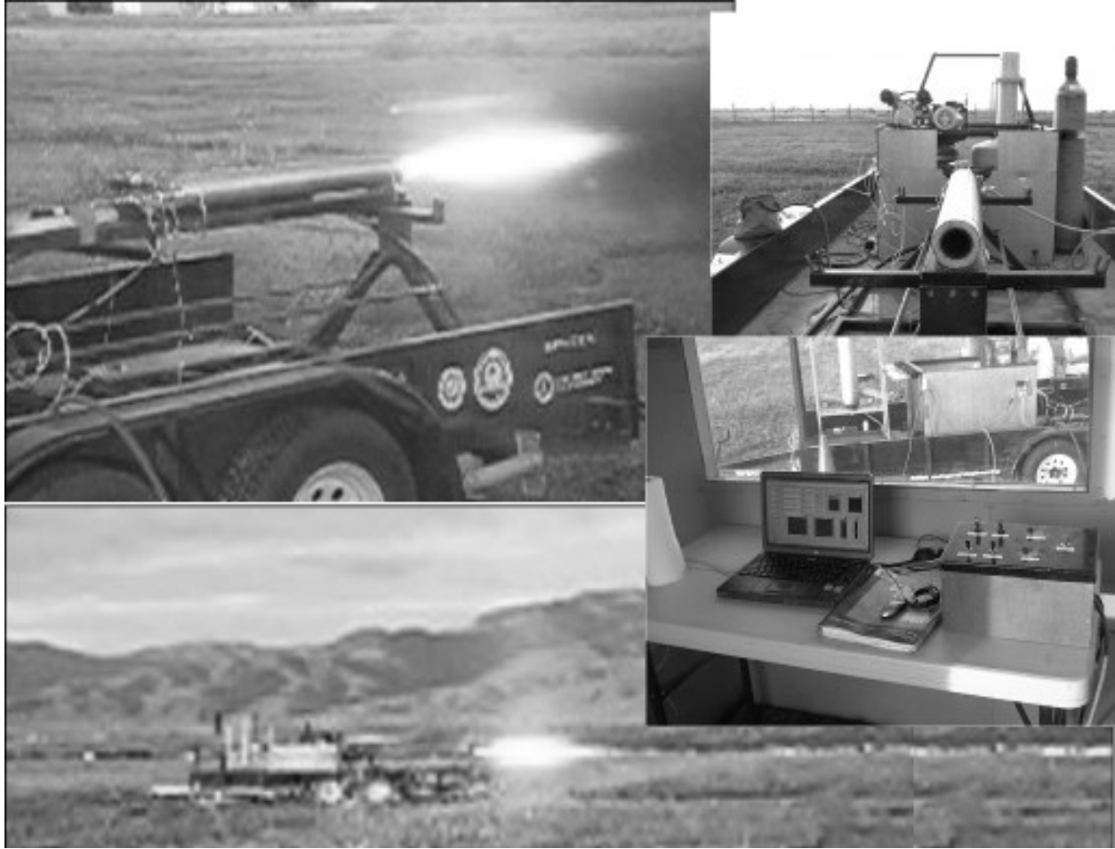
Figure 6. Typical test firing of a 4 in nitrous oxide and HTPB hybrid rocket motor.
