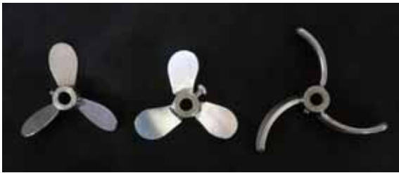
Fig. 2 Photograph of propeller and pfaudler type impellers
