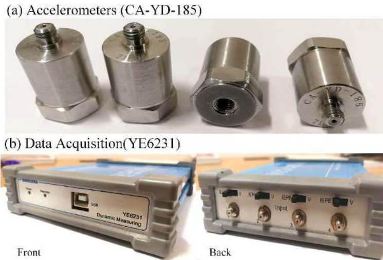
Figure 8 Accelerometers and data acquisition system
