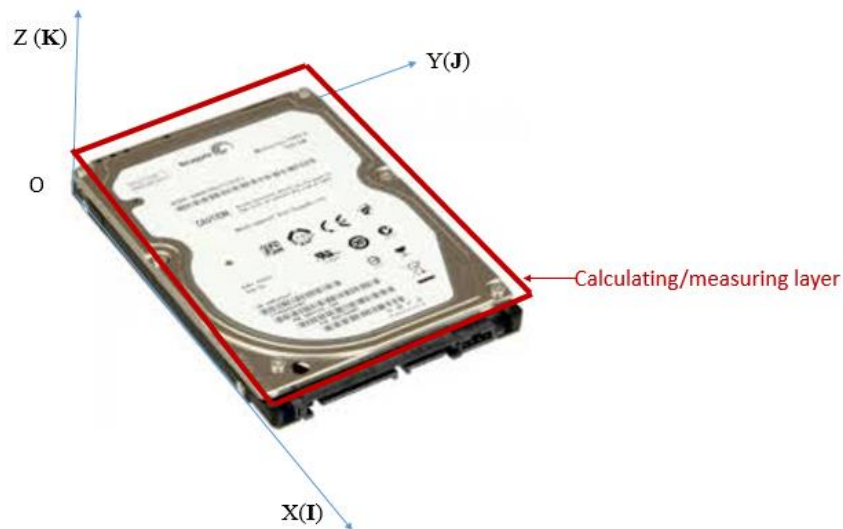
Figure 3-1 Near field calculating/measuring layer for 2.5" HDD
