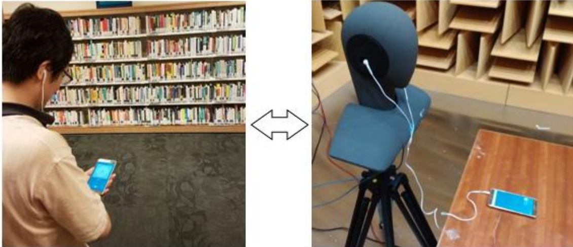
Figure 2-10 A typical example of participant taking Jury Test 1 in the library (Left) and sound recording setup for playback system in acoustic chamber (Right)
