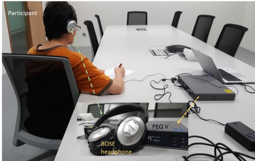
Figure 2-15 Participant taking Jury Test 2 and HEAD Acoustics equipment
