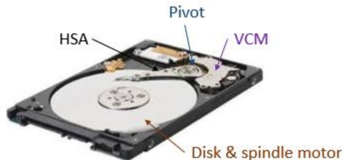
Figure 1-3 Typical 2.5" HDD interior
