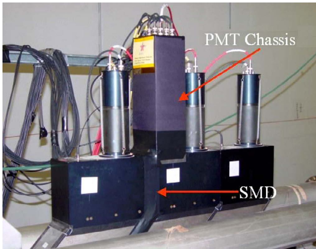
Figure 4.4: A ZDC-SMD module shown installed at STAR.
