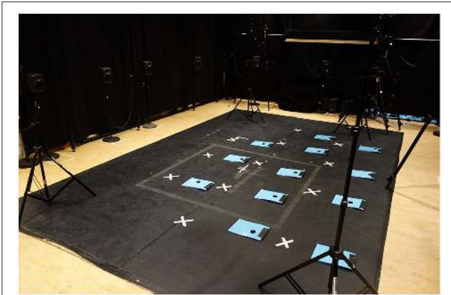
FIGURE 2 | The setup for the experiment in the motion capture laboratory. White marks and questionnaires indicate the position of each participant. Poles with reference markers were placed in each corner of the capture space and used to check the noise-level of the recording (see Jensenius et al., 2012 for a description of the noise-level in optical motion capture systems).
