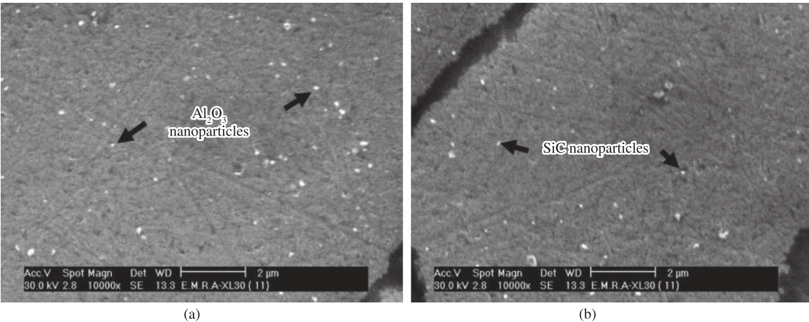
Figure 4. SEM micrographs of a) Al/3 vol.% Al 2 O 3 (60 nm) and b) Al/3 vol.% SiC (200 nm) nanocomposites.
