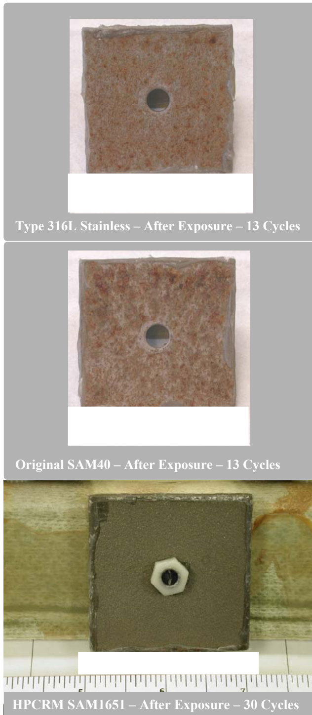
Figure 10 – Early thermal-spray coatings of Type 316L stainless steel and the SAM40 parent material showed relatively severe corrosive attack after only 13 cycles in the ASTM B117 salt fog test. However, several of the new Fe-based amorphous metal coatings, including SAM1651 and SAM2X5, have shown no corrosion, even after more than 30 cycles in this aggressive environment. It is therefore believed that these new materials will provide substantial benefit in some Naval applications.
